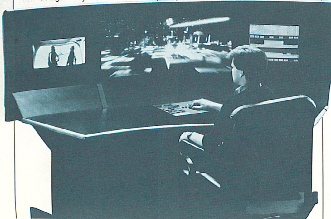
EditDroid's control console. Control panel on table in front of editor controls functions. Electronic log sheet is displayed on right hand screen; raw footage on left screen and cuts are displayed for approval on central monitor.
