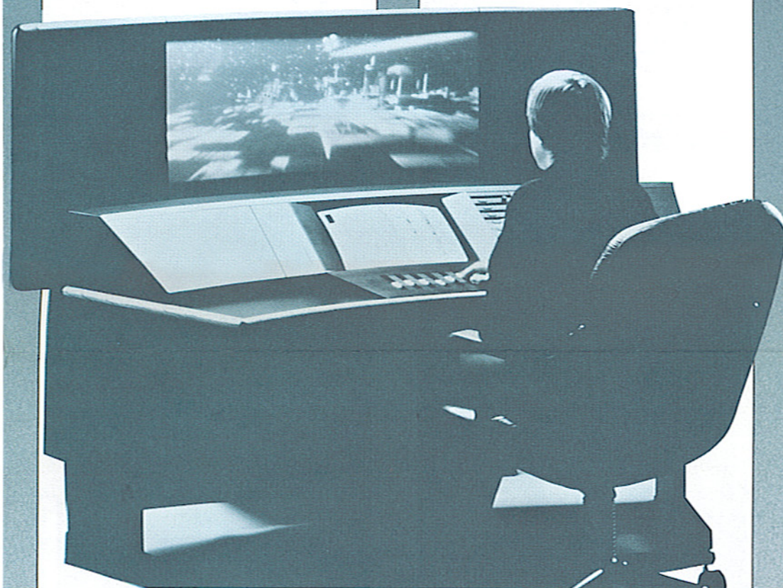
SoundDroid's control console. The editor can watch the scene to which he or she is adding sound. In front of the monitor screen is the electronic cue sheet with a slide pot (potentiometer/volume control) for each track.
